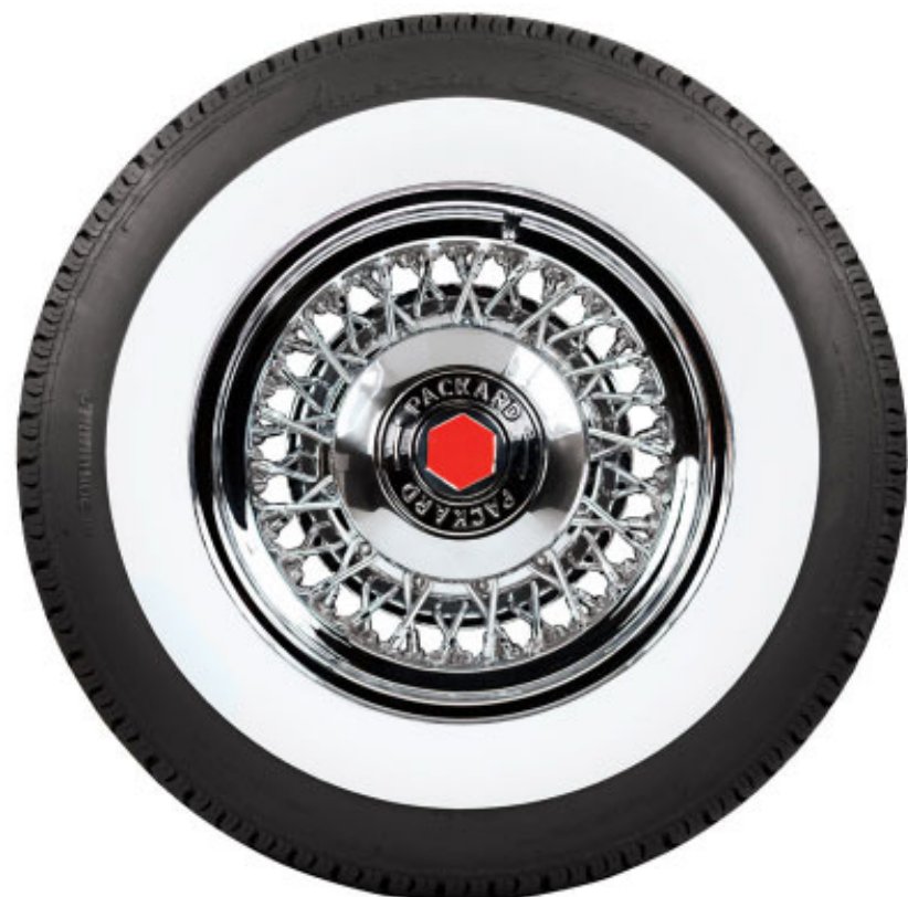
15 X 6" wire wheel with 56 spokes - larger sizes available
