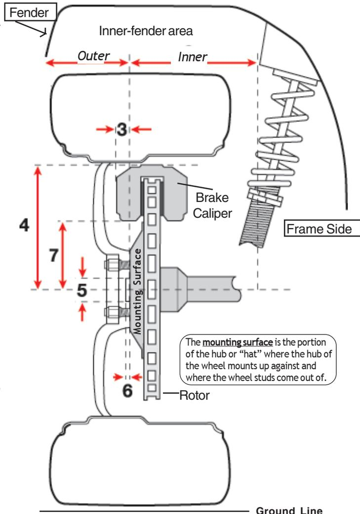
The **mounting surface** is the portion of the hub or "hat" where the hub of the wheel mounts up against and where the wheel studs come out of.
