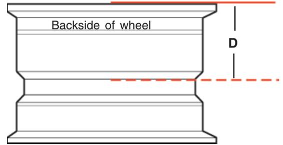
Side view of wheel with back side up. Lay your wheel down to measure. Measure with a straight edge **across the back lip of the wheel.**
