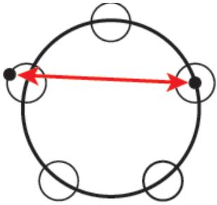
**(A) Begin by measuring your bolt pattern.** Note how you measure from the center of one hole to the outside or furthest edge of the hole diagonally across from it. The measurement is: \_\_\_\_\_"
