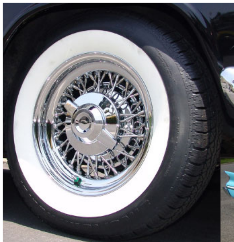
Shown above: 15 X 6" Truespoke wire wheel with P235/75R15 American Classic whitewall tires. Whitewall size: 31/8"
