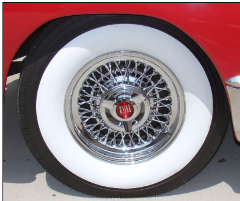
Above: Buick wheel and tire package. Tire size: L78-15 with a 4" whitewall
